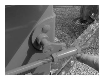
In order to adjust the chain control arm, use a 3/4" wrench to loosen the nuts on either side of the slide tee, (located on the front of the control rod). Move the control rod to the front or rear as needed, and re-tighten the nuts. The adjustment is complete when the control arm lifts the chain from all of the teeth in the drive gear. You may have to repeat this adjustment several times in order to achieve the proper setting.
