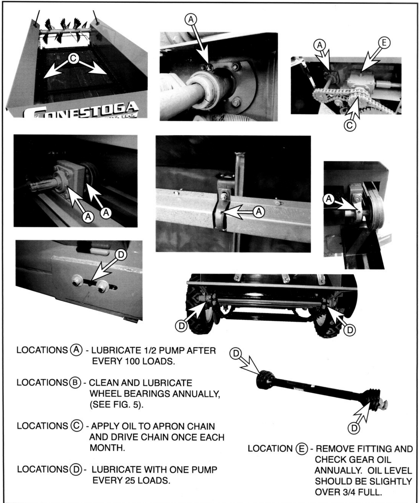
FIG. 5 - LUBRICATION REQUIREMENTS (ALL PTO MODELS)
